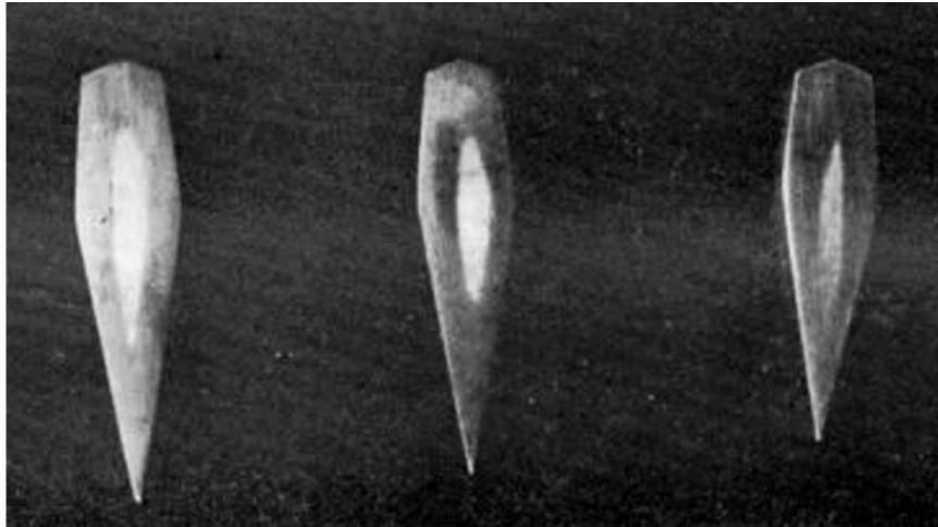
Fig. 3 - Sections of Koa Isshin blades, as shown in the book about Koa Isshin. It is shown here how the shingane is correctly positioned inside the kawagane.
